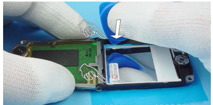
Remove LCD Module by using SRT-6 as shown in the picture.
