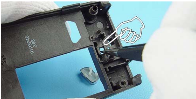
The Release Key can be removed by pushing with tweezers through the opening in C-Cover.
